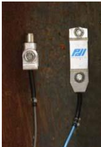
Figure 2.9. Strain gauge and accelerometer attached to a pile for dynamic testing (GRL Engineers, Inc. 2014)
